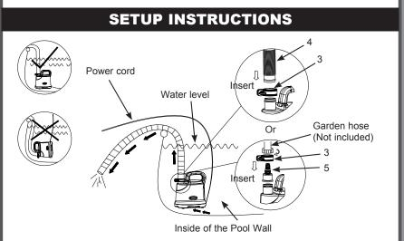
**NOTE:** Maximum pool **water depth** not to exceed 48 in (1.22 m). To protect the pump motor from running dry, disconnect the power cord from the electrical outlet once the water has been drained out or when the remaining water is below the drainage pump base.
