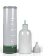
As soon as the liquid has turned green, you have determined the hardness of the water using the amount of drops added.
