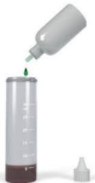
As long as the water is red, add the liquid drop by drop into the measuring cup. Count each drop and shake the measuring cup after each drop.
