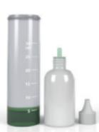
As soon as the liquid has turned green, you have determined the hardness of the water using the amount of drops added.
