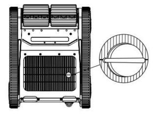
② Remove the plug cover. When fully charged, cover the plug again.
