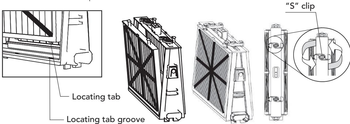
Reinstall the base frames with filters according to the diagram.
