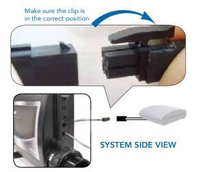
After the Gateway Ultra Spa module is inserted, gently pull on the wire to make sure the clip is securely in place and will not come lose.
