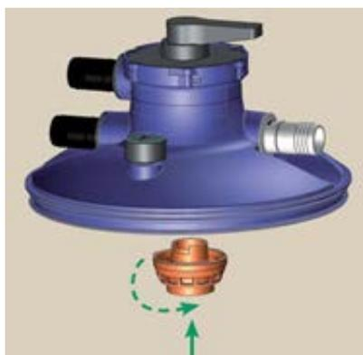
Centre the diffuser in its housing, and push it firmly against the lid, twist it to slide the tongue of the diffuser fully into the U shaped groove in the lid.
