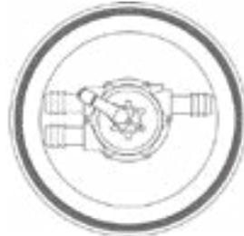
**BACKWASH:** Water from the pump crosses the filter from the bottom to the top and is then routed to waste taking with it dirt and debris trapped by the filter.
