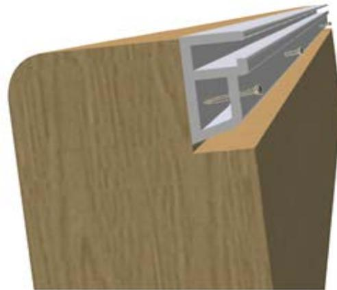
Figure 26 – Installing the liner locking track
