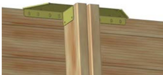
Figure 18 – Fastening metallic support brackets to the top of the supporting braces
