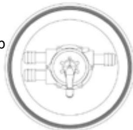
**DRAIN:** Water from the pump passes directly to waste without passing through the filter.
