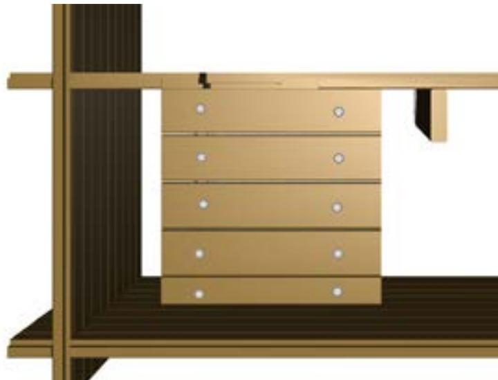
Figure 15 – Assembling the base of the plant housing portion of the box
