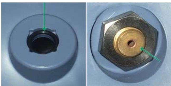
Place the o-ring in its groove in the lid. Orient the pressure gauge and place it in its housing.
