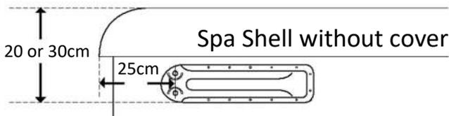
Adjust the mounting position according to cover length/width, cover thickness and spa corner radius.
