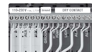
AUX 1 1 & 4 Base (pump) or Ultraviolet (according to model) AUX 2 5 & 6 redoX / Free Chlorine ppm's (pump) AUX 3 15 & 14 AUX 4 15 & 16 Heating control
